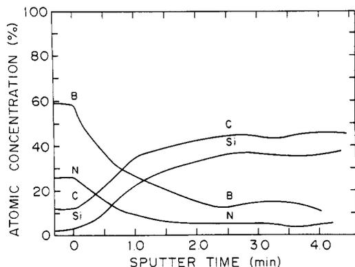
**Figure 9.** AES depth profile of Nicalon SiC fibers that have been dip-coated in  $\sim 0.1$  M (2% w/w) solution of  $(\text{CH}_3)_2\text{S}\cdot\text{BHBr}_2$  and pyrolyzed under  $\text{NH}_3$  to 1000 °C.  $\text{Ar}^+$  sputtering rate = 125 Å/min.
